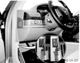
Note: When using an OBD scan tool for diagnosis, the transmission speed is 10.4 KBit/s.
